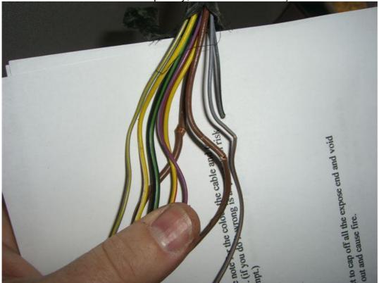
Now I retired all the cables from the interior and voila: 4 cables had a problem! (1 came off completely, 3 had a severe cut):
