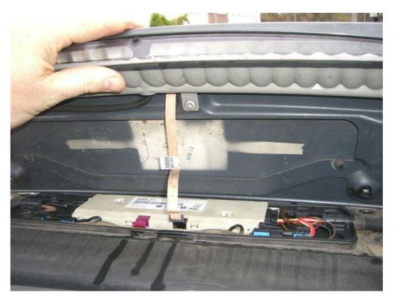
I removed this antenna cable, and on the right hand side I unplugged the high breaking light connector:
